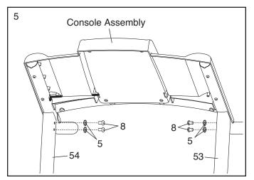
6. Start an M8 x 15mm Bolt (8) with an M8 Star Washer (5) into each Upright (53, 54). Then, firmly tighten all six M8 x 15mm Bolts (8).
